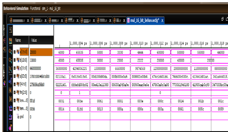
Fig. 12: 16x16 Braun Multiplier Simulation waveforms
